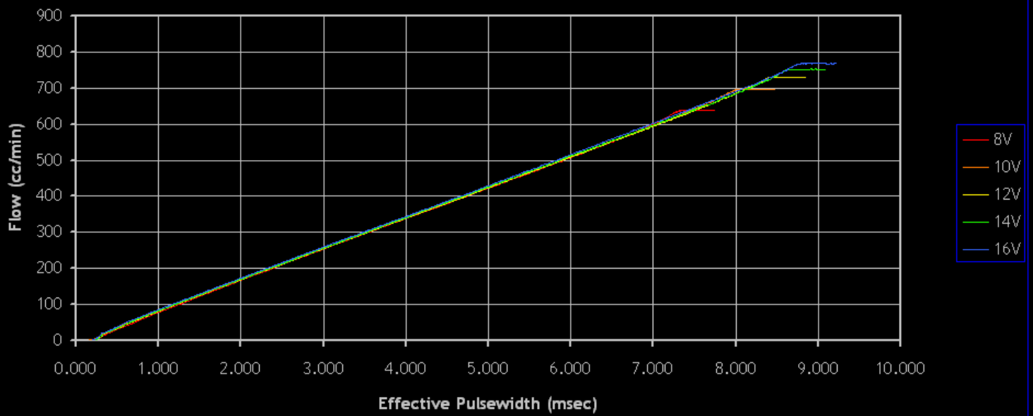
Injector Dynamics ID725 Corrected Flow @ 4.14 Bar
