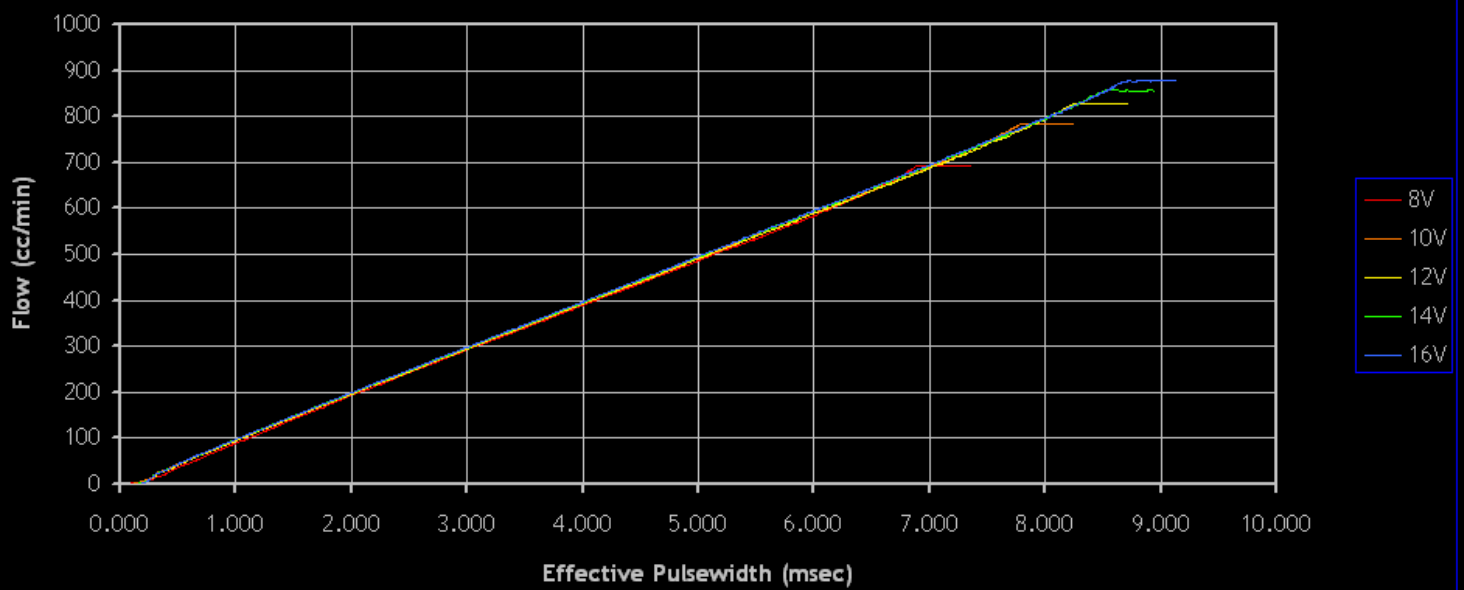
Injector Dynamics ID725 Corrected Flow @ 5.52 Bar
